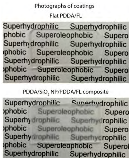
Figure 8 | Photographs of flat and optimized layer-by-layer composite coatings. The flat coating appears transparent suggesting any reduction in transparency for the composite coating is due to the SiO 2 nanoparticle layer.
