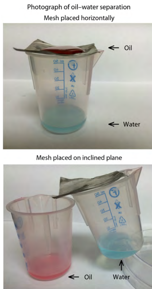
Figure 9 | Photograph of optimized layer-by-layer composite coated stainless steel mesh acting as an oil–water separator. The superoleophobic/superhydrophilic nature of the coating results in water passing through the mesh while the hexadecane oil remains on the top surface of the horizontal mesh and can be easily rolled off. Alternatively the mesh can be placed on an inclined plane and oil and water collected simultaneously in separate beakers. Oil and water dyes used to enhance contrast.
